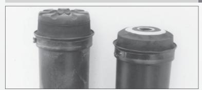
Remove stock dust boot and modify using a grinder or delete (See Photo). If strut was removed, re-attach to spindle now.
